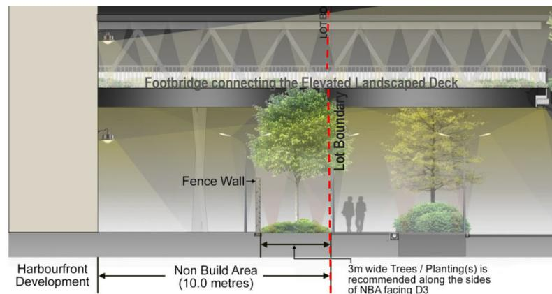
**Figure 4.32** The diagram above shows the distribution of light when wide-angle lights which are not recommended are used. A considerable amount of light is wasted. Residents of buildings near the road / footpath would suffer from light trespass and must keep their curtains etc closed to tackle excessive and unneeded illumination of their windows.
