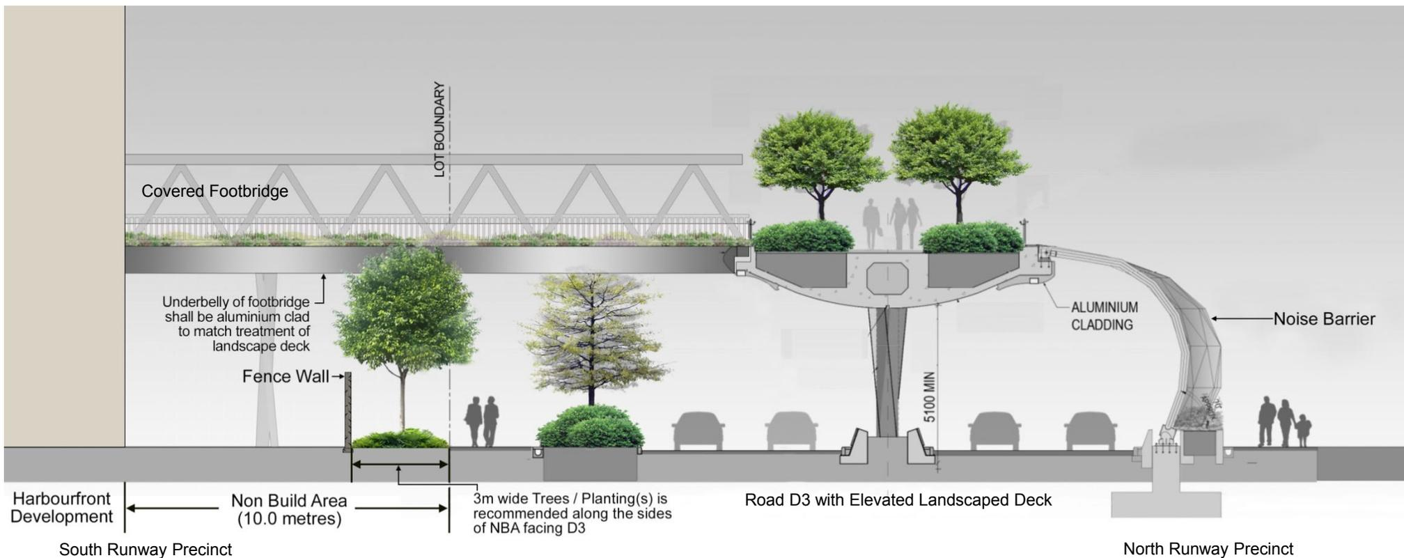
Figure 3.28 Arrangement of footbridge connection from harbourfront development to landscaped deck
