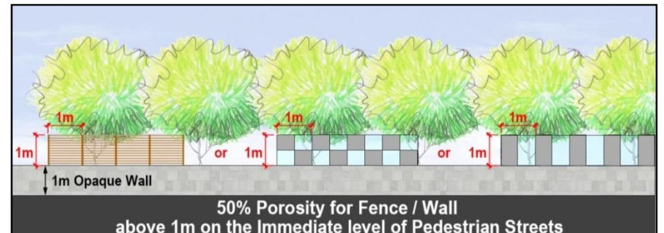
Figure 4.17 Typical fence wall setting out detail
