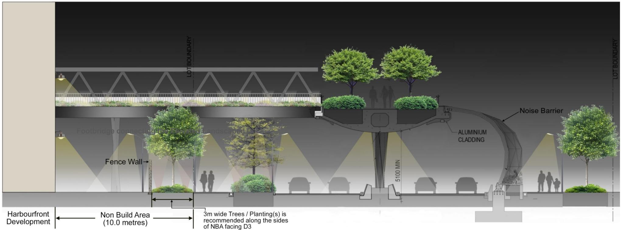
**Figure 4.33** The above illustration indicates that uniform focussed lighting is vital to reduce glare. The selection of lighting applications and treatments needs to focus on avoidance of glare and lighting spillage.
