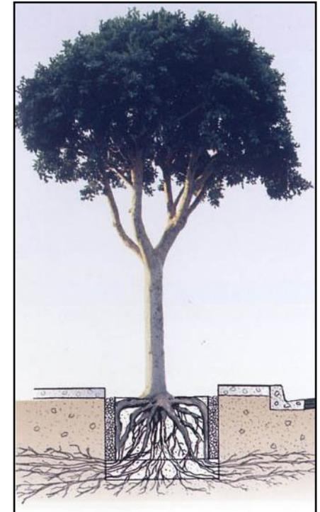
**Figure 4.35** Root control barriers can effectively limit root intrusion and should be used extensively in the public realm
