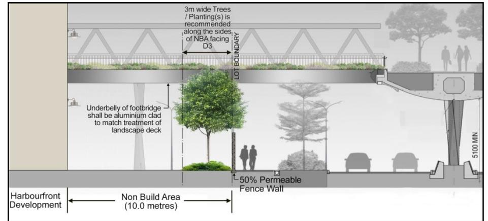
Figure 3.79 Example of acceptable standard planting and fence wall arrangement for NBA abutting Road D3
